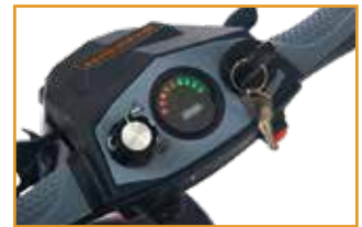
LED battery indicator on the console
